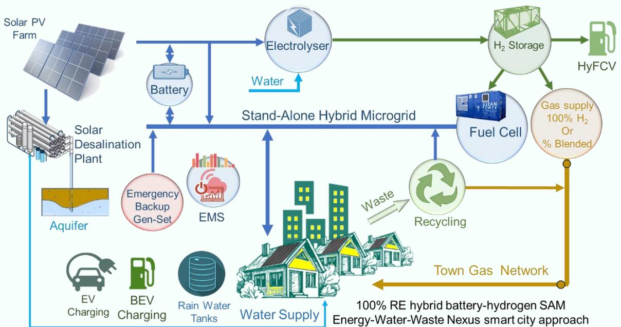
Figure (B1): Proposed 100% RE hybrid battery-hydrogen SAM system model
