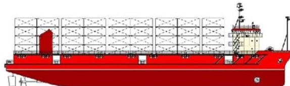
Figure 21: Small RORO vessel suitable for a mix of containers and break-bulk cargo
