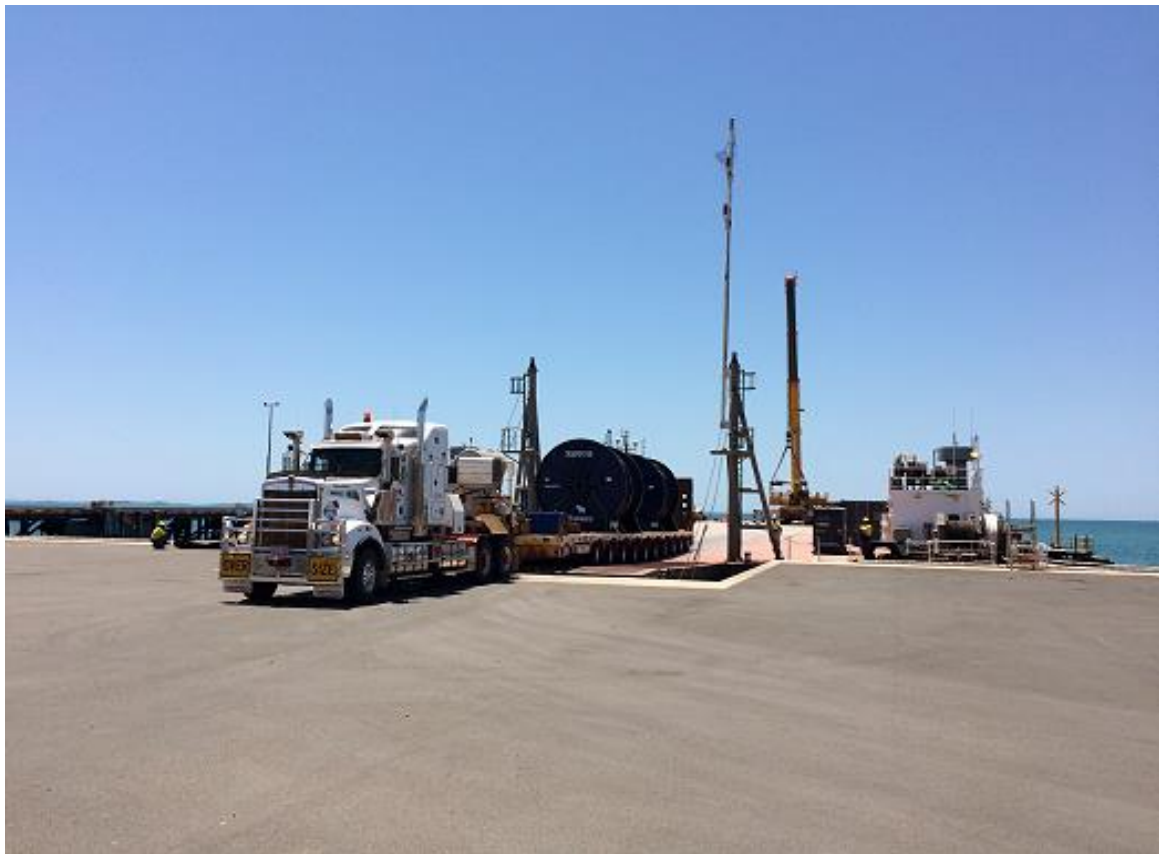
Figure 18: Heavy RORO cargo discharged from a trans-shipment barge at the FDTS berth
