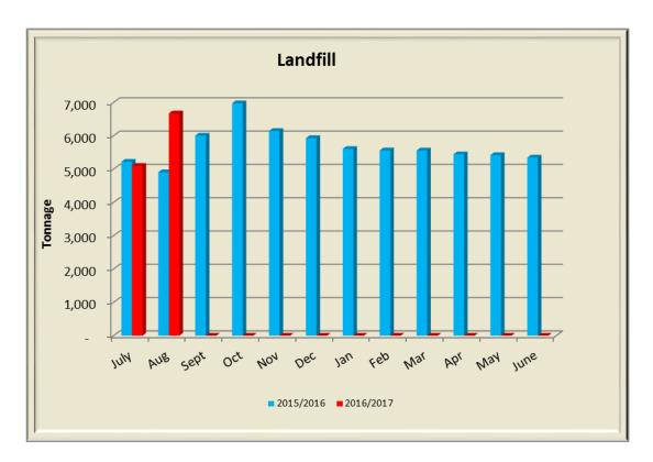
Total waste, excluding liquid and clean fill delivered to the 7 Mile Waste Facility. Approximately 1500 tonnes of Contaminated Soil was delivered to 7 Mile in August.
