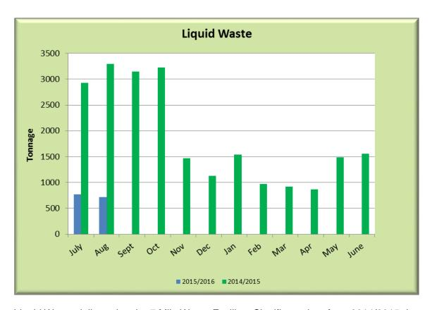
Liquid Waste delivered to the 7 Mile Waste Facility. Significant drop from 2014/2015 due to Karratha Environmental Crushing commencing operation of liquid waste ponds and the reduction in camp utilisation.
