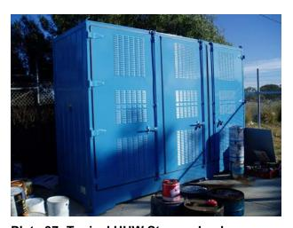
Plate 37: Typical HHW Storage Locker Lockable storage locker at Henderson Landfill for the storage of household hazardous waste.
